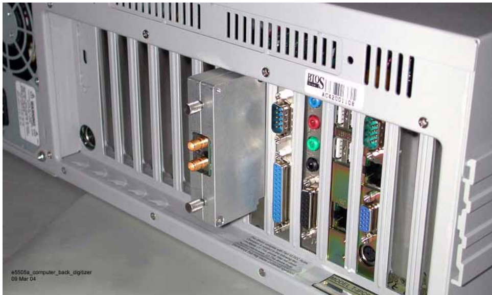
Figure 317 Connect adapter to PC digitizer card
